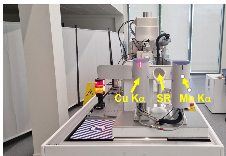
Figure 11. The exemplary view of the SAXS system connected to two X-ray tubes (Cu K \alpha , Mo K \alpha ) and with open port for synchrotron radiation.
