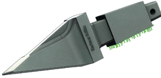
Fig. 8. Fixation conditions of cutting tooth
