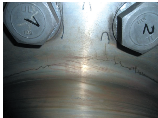
Fig. 3. Cracks on circumference and radial cracks [1]
