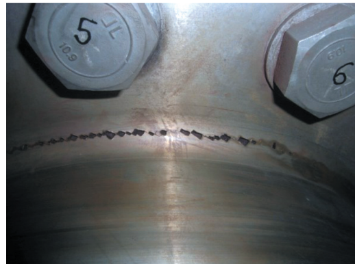
Fig. 2. Cracks in circumference with crushing [1]
