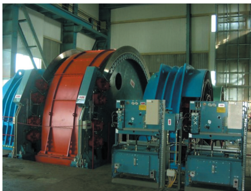
Fig. 1. View of hoisting machine in section (S) of R-II shaft after modernization in 2004 [1]
